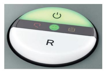
Advantage: Our shredders offer convenient operations via EASY\_SWITCH. This multifunctional element has integrated optical symbols for the operational status.
