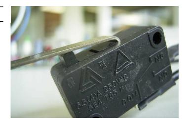
**Danger:** Easily jamming switches which are not protected against paper dust.
