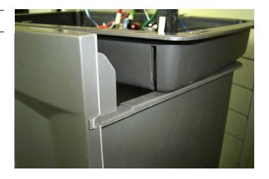
Danger: If the machine head is taken off or the door is opened, the shutdown system can be easily manipulated.
