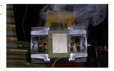
Danger: Cheap shredders are equipped with motors which may overheat. There is no thermal protection.
