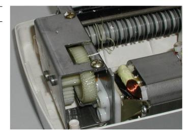
Disadvantage: Open gear-box. Low quality gears which are causing noise and wear out quickly.
