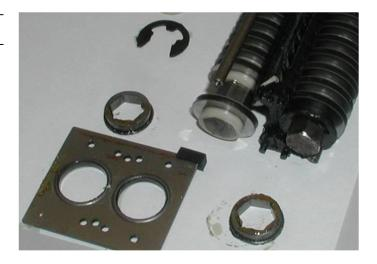
**Disadvantage:** Simple cutting knives just put on an axle. Strong wear and tear of cutting shafts – metal is not hardened.
