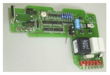
**Safety:** PC-boards coated from both sides. Strong, reliable plugs. By using transformers, the voltage on PC-board is only 12 volt.
