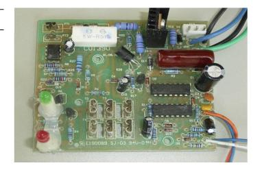
**Danger:** PC-boards coated only from one side. Weakly soldered cables. Dangerous high-voltage on the PC-board!
