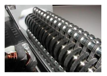
**Advantage:** Our cutting shafts are made of one single piece and of special hardened steel. Outstanding know-how for perfect geometry.
